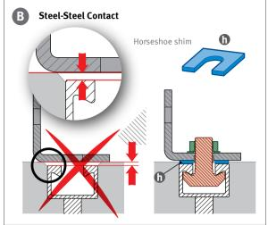
A defined contact must be produced between channel and attached component.
