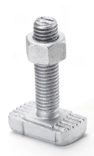
All JORDAHL® T-bolts are purpose made to ensure reliable and accurate connection with the range of JORDAHL® channels. The T-bolts face enter into the channel profiles and rotate 90 degrees to safely lock in position. Lines on the end of the T-bolts indicate the head position for easy checking after installation.
