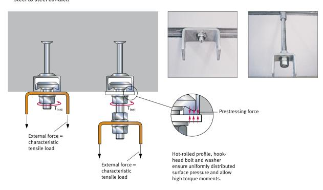
The relationship between prestressing force and tightening torque are shown in the graphs below. The prestressing forces vary strongly with the friction in the thread between the nut and the T-bolt. Low friction causes high pre-load, typical for hot-dip galvanized T-bolts with lubricated nuts.
